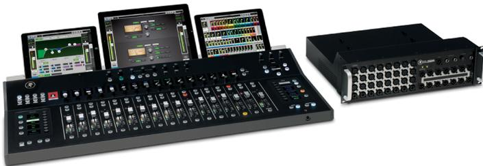
We need to do this one component at a time. When updating the DC16, the DL32R will need to be turned off. Likewise, when updating the DL32R, the DC16 will need to be off.
