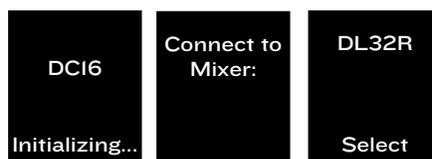
The DCI6 screens will show a list of the 4 DL32R “slots” to connect to. Press the encoder under “Slot 1, FOH”.
