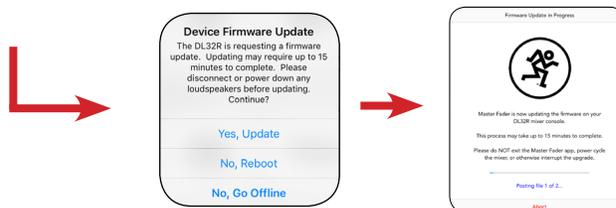
This update will take up to 15 minutes. It is complete when the Master Fader “Updating Firmware on your DL32R” prompt disappears, and connects to the DL32R showing a green dot in the Master Fader Tools (gear) icon.
