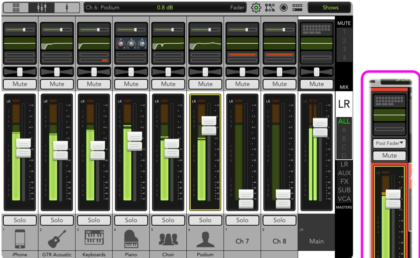
Remember, the LR mix levels are controlling the Aux mix so if you need to turn down the Aux mix just turn down the Aux master accordingly.
