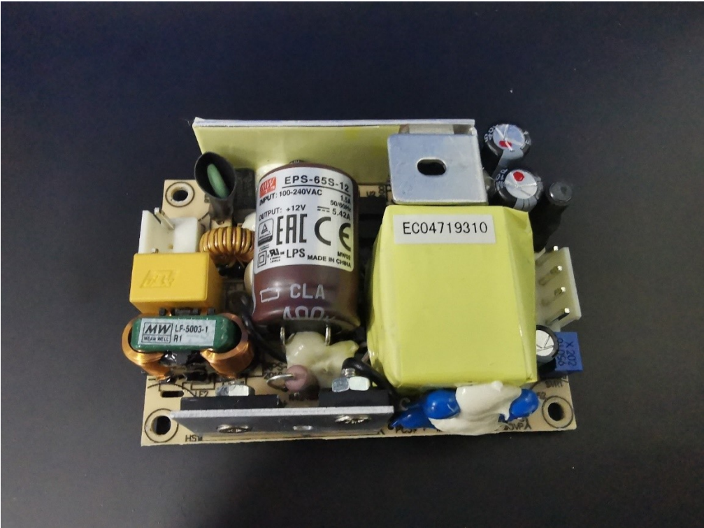
Component side view of internal power supply board EPS-65S-12
