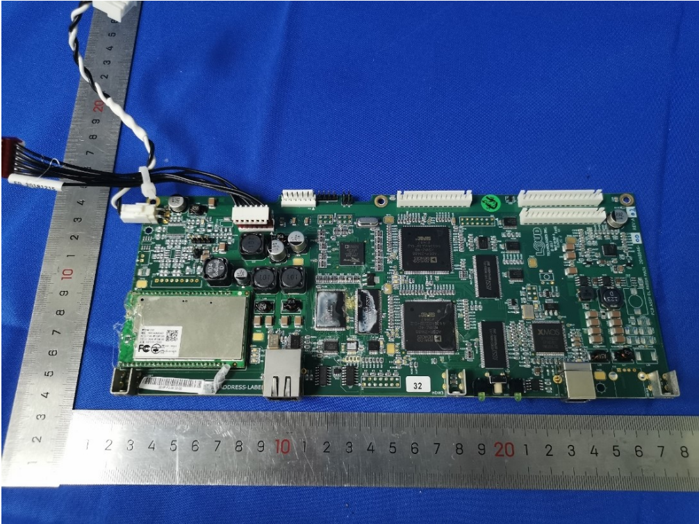
Component side view of main board for model DL32S
