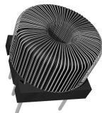
This little bitty thing, discussed below, is the bifilar-wound dc pile transformer that makes the huge difference in XDR sound quality.
