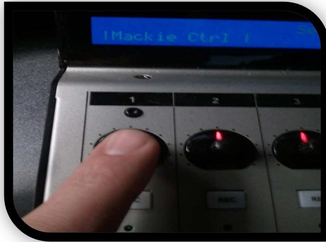
5. Once in Mackie control mode, you can press buttons and notice the corresponding LED illuminate. That means the unit is sending and receiving its own midi message. See example photos below:
